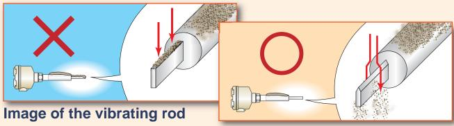
If the sensitivity is high, the output will not turn off when the material remains on the rod.
