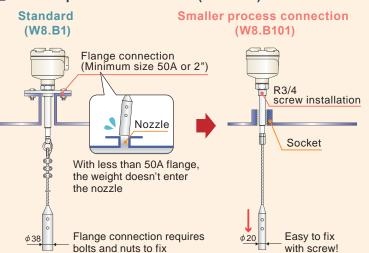
$\odot$  Chain weight  $\sim$  When measuring solid lump  $\sim$
