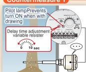
Since it hits the main electrode intermittently, it prevents the switch from turning on immediately by delaying the time.
