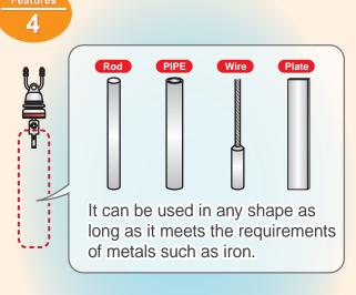
A wide range of detection electrodes can be selected, such as wire and steel.
