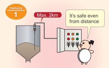
The maximum wiring between the detector and the amplifier is 2km.
