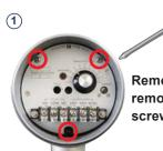
Remove the case cover and remove the amplifier fixing screws indicated in 3 places.
