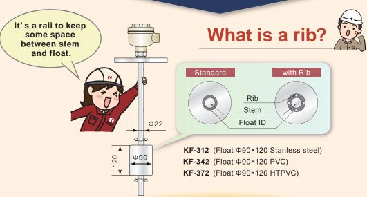
Rib prevents float malfunction caused by surface tension orbiting solid.
